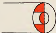
FIG. 2 NODAL PLANES (TWO CYLINDRICAL, ONE PLANE)
