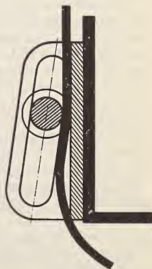
FIG. 2b GRIP-ROLLER LOCKING DEVICE FOR A BELT
