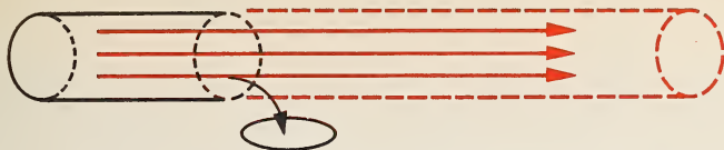
FIG. 1 TRANSFORMATION OF CAVITY RESONATOR INTO WAVEGUIDE
