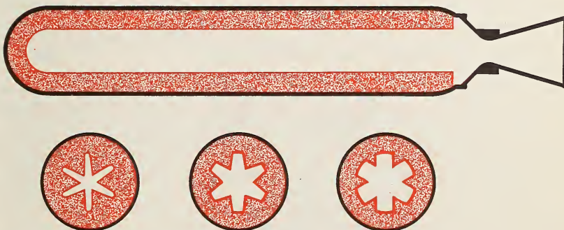
FIG. 2 LARGE SOLID-PROPELLANT ROCKET MOTOR WITH STAR-SHAPED CAVITY
