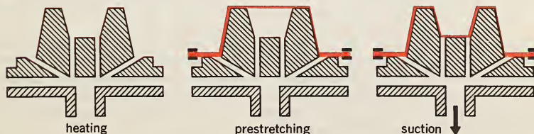
FIG. 9 VACUUM PROCESS: POSITIVE-MOLD METHOD
