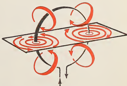
FIG. 4 MAGNETIC FIELD OF A CIRCULAR CONDUCTOR
