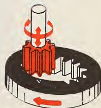
FIG. 2c PINION-CUTTER PROCESS APPLIED TO INTERNAL TEETH
