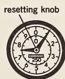
FIG. 3 TWO-POINTER DIAL MECHANISM
